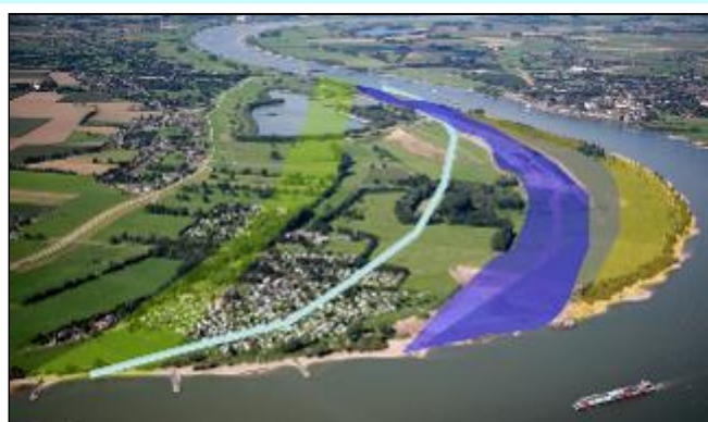
Figure 2: Five alternatives for the spillway and lowering the floodplain
